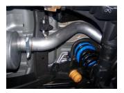
**4.** Install overaxle tailpipe #C into muffler. Insert welded hangers into rubber grommets.
