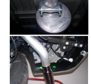
6. Install stainless steel tip #D. Clamp down. When you have everything in place, firmly tighten all bolts and clamps down securely. Use stainless steel cleaner and a Scotch Brite pad weekly to prevent tip from discoloration. Inspect all fasteners after 25-50 miles of operation and re-tighten as necessary.
